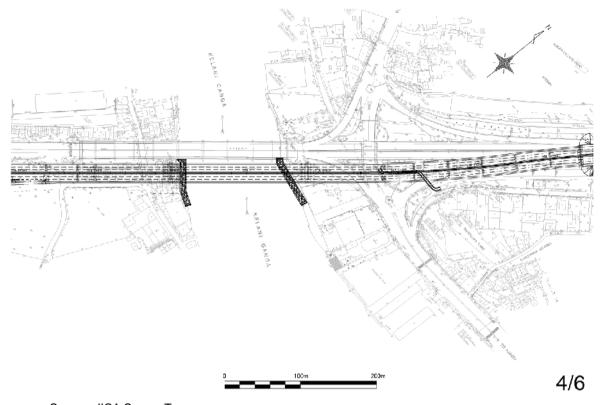
Figure 3-5(4) Access Road during Construction Period
