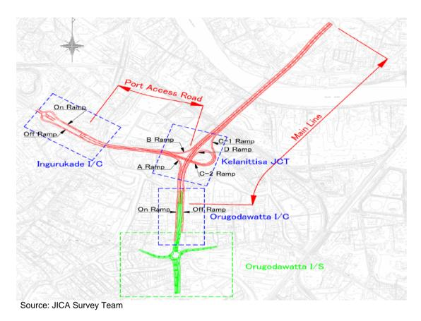
Figure 3-4 Main Structures to be constructed in the Project
